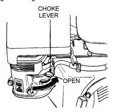
Figure 8. Engine Choke Lever (Open)
